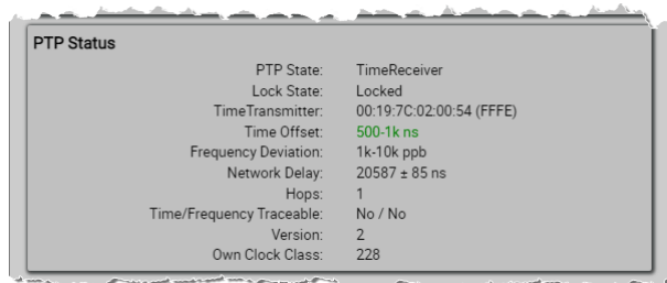
Figure 68: Info (Antennas) – PTP Status (e.g. DECT Antenna in Standalone/AES67 mode)
